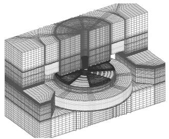
Fig.2. DC60 finite-element model
