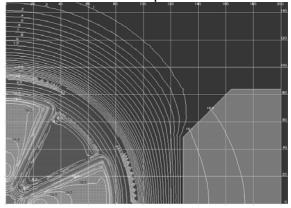
Fig.5. Simulated field map in DC60 median plane.
